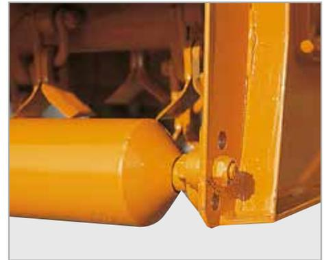
Adjustable rear roller - simple cutting height setting.
