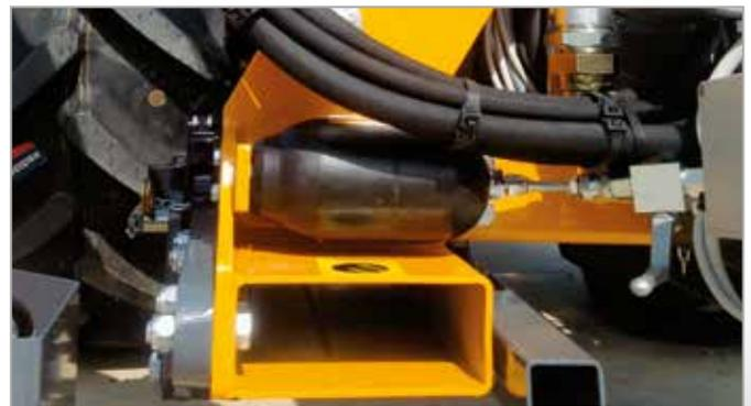
Optional lift float accumulator allows smooth operation with reduced bounce on the arm.
