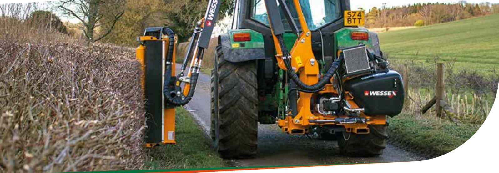
The **T500G AND TPE600** are the flagship models of the Wessex hedge cutting range. Both feature a 1.2m working width head with the option of various flail types for different applications.
