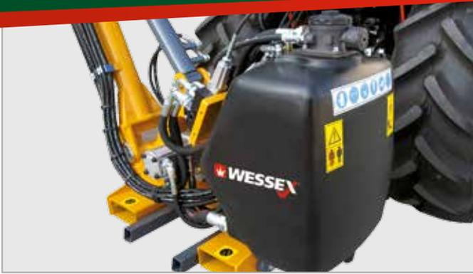
The polypropylene oil tank is separated from the frame which allows it to be isolated from any structural stress. Fully recyclable.
