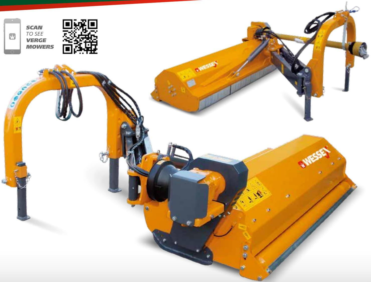
The **WESSEX ZMTE** is a popular general purpose verge mower in 3 working widths from 1.6m to 2.0m. Ideal for use on estates and within the agricultural market sector, the ZMTE features a side mounted gearbox, adjustable rear roller, the option of a hydraulic break-away device and the choice of Y-pattern or hammer flails.
