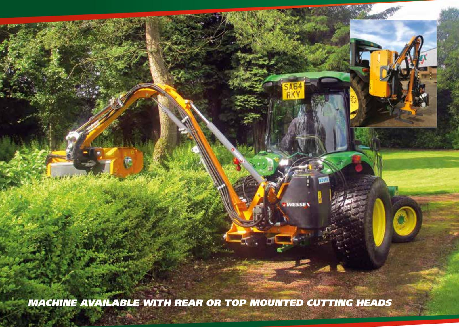
**MACHINE AVAILABLE WITH REAR OR TOP MOUNTED CUTTING HEADS**
