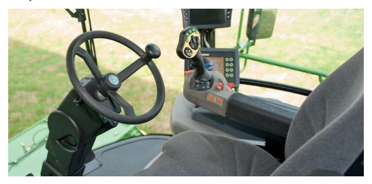
BiG M 500 features four-wheel steering as standard specification. The operator can choose between various modes.
