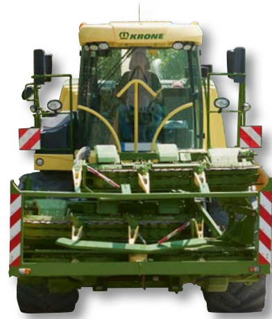
Compact transport width: the three-section EasyCollect
