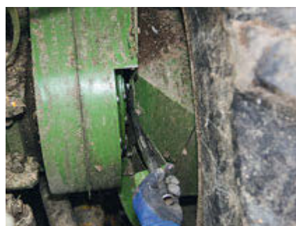
The VariLOC speed is changed with a regular 36mm spanner.
