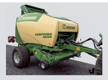
and maintain than a variable chamber round baler. It produces bales of various diameters by building the pressure from outside and the bales have a very small and soft core at larger diameters and as a result are heavier in weight.
