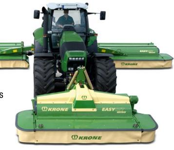
to the absolute minimum, whereas you want wider overlaps and a narrow work width when you are cutting around bends. As you operate on the slope, simply retrieve a stored sideshift range to the right or left and avoid drifting and striping.
