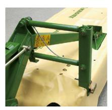
Spreading the load: The parallelogram linkage absorbs the lateral forces and guides the unit in direction of travel. At the same time, it helps reduce the load on the jib and the center-of-gravity suspension system.
