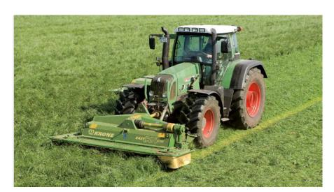
EasyCut 28 CV front-mounted disc mower
