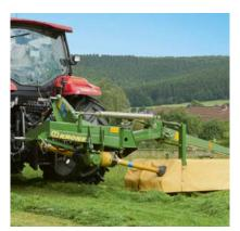
Uniform speeds: The direct drive system, which relies on driveshafts and gearings, provides positive drive in heavy crop and at wide working widths. 1,000 rpm gearboxes are available as optional extras to suit a 1,000 rpm pto.
