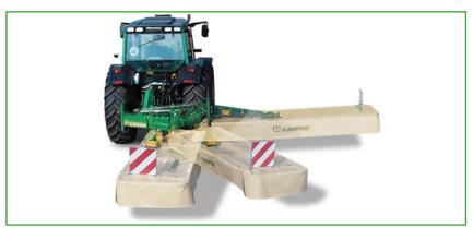
Hydraulic changeovers from transport to work and vice versa: A double acting ram swings the mower into position. The system offers straightforward and convenient control from the cab via a double acting spool. Low in profile when in park position, the mower is transported at a generous ground clearance.
