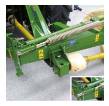
Adjust the ground pressure conveniently to requirements. Easily adjustable coil springs provide quick and optimum adaptation to all conditions. The kinematics between the coil spring and the main beam maintain a nearly consistent ground pressure, even in undulating terrain.
