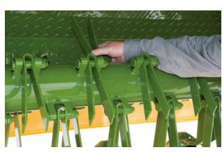
V-type pivoting steel tines and a steplessly adjustable baffle plate provide uniform crop treatment, reduce machine wear and optimise adaptation to crop conditions.
