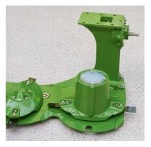
No inner shoe: The cutterbar is powered via a right-angle gearbox, which is arranged immediately behind the inner top hat, a design that ensures blockage-free operation on the headland and in awkwardly shaped fields.
