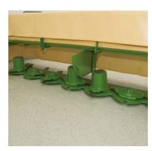
Flexible: EasyCut 400 features top hats in the middle which form two windrows that the tractor can straddle. You can replace these top hats by discs, if spreading and faster wilting is the aim.
