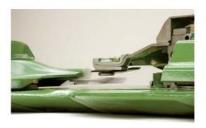
Unlimited spinning: The knives are free to spin through 360°. They are hardwearing and self-cleaning, well protected and will not foul with the knives on the neighbouring discs.
