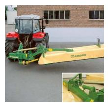
Convenient: a hydraulic ram raises the machine on the headland. Linked to the ram that swings the unit in and out, this ram also provides for impact damage protection, as it instantly lifts the machine the moment the break-back system trips.
