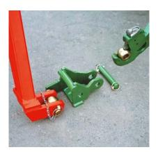
The perfect match: KRONE offers adapters to fit into rigid lower link arms and a telescoping top link extension, which enable transverse ground tracking.
