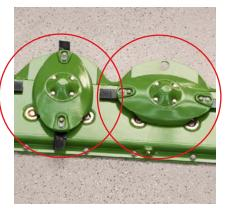
Excellent cuts - 112 mm (4.4") knives mount on their individual discs in alternate arrangements, giving generous overlap. Impact stops are welded between the skids to protect the cutterbar from damage and deliver an excellent cut.
