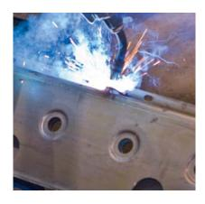
Rugged and absolutely leak-free: KRONE cutterbars are fully welded by advanced robot and CNC systems to meet the most exacting demands and quality standards. After all, the cutterbar is the heart of every disc mower.
