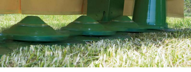
The wedge-shaped cutterbar gives EasyCut the edge for better cuts – short in pastures and slightly longer in long-stemmed field crops. The wedge-shaped design provides a greater choice of settings and more options to deal with difficult conditions. As another KRONE advantage, the massive spur gears run in double bearings, which in turn are spaced wide apart to withstand high and permanent loading. The hardened
