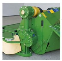
The conditioner shaft is powered by a twospeed (600rpm and 900rpm) mechanical gearbox which forms an integral part of the driveline.
