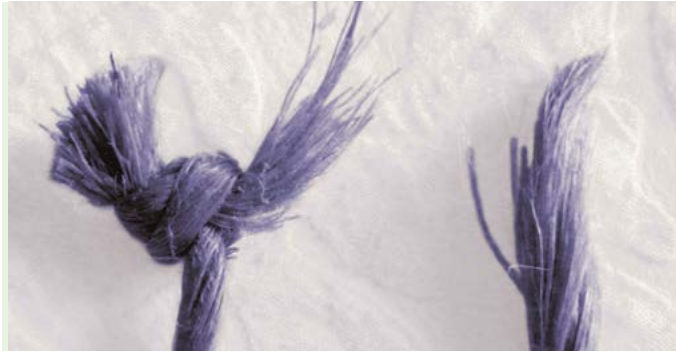
The strain is highest in the knot. If knot strength is low, the twine will most likely tear here.
