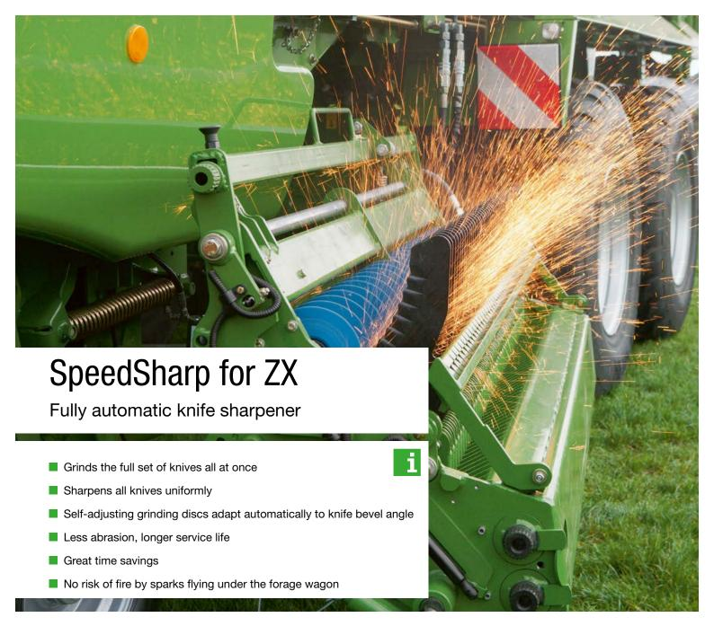
SpeedSharp is a fully automated knife grinder for the cutting system on the KRONE ZX dual-purpose forage wagons. The sharpener is made up of 23 grinding discs that are arranged on a hydraulically powered shaft which grind the full set of 46 knives in only two passes.
