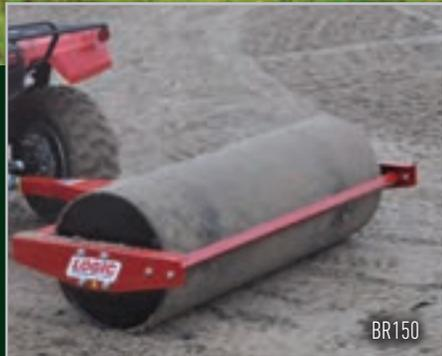
Adjustable scraper to prevent mud build-up on the barrel in damp conditions.
