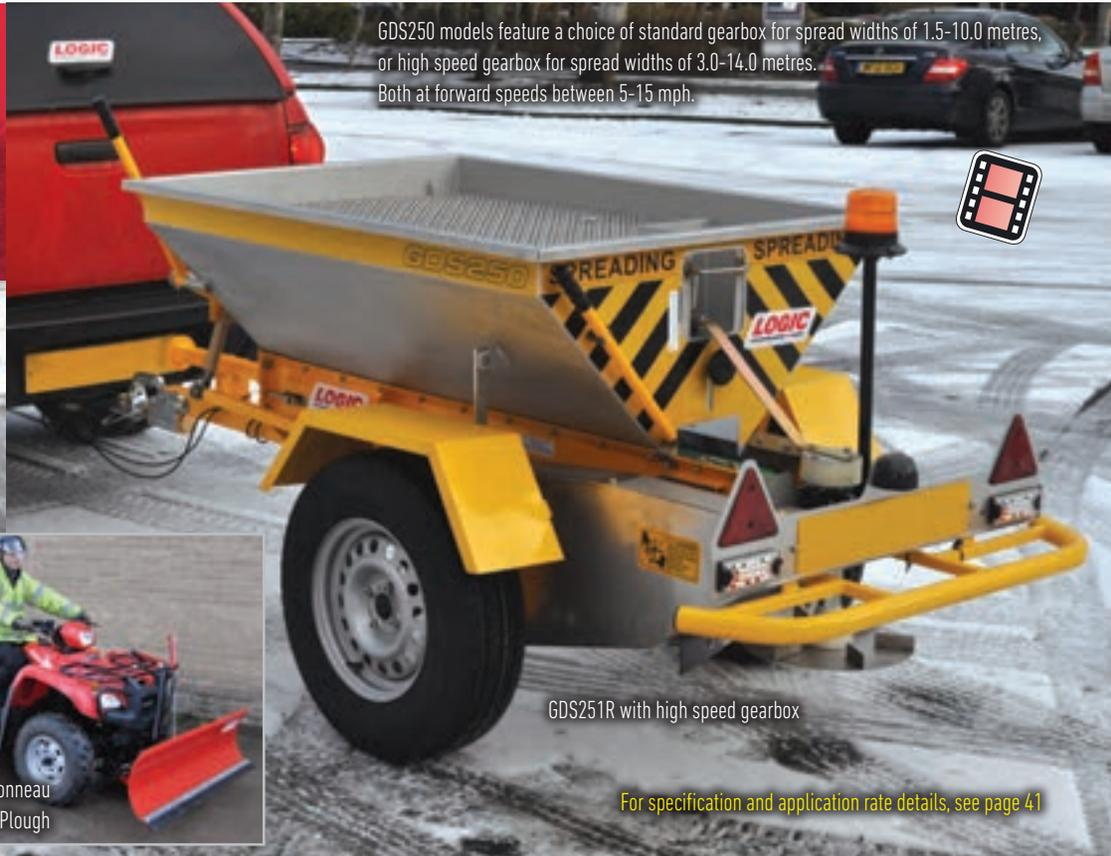
GDS250 models feature a choice of standard gearbox for spread widths of 1.5-10.0 metres, or high speed gearbox for spread widths of 3.0-14.0 metres. Both at forward speeds between 5-15 mph.
