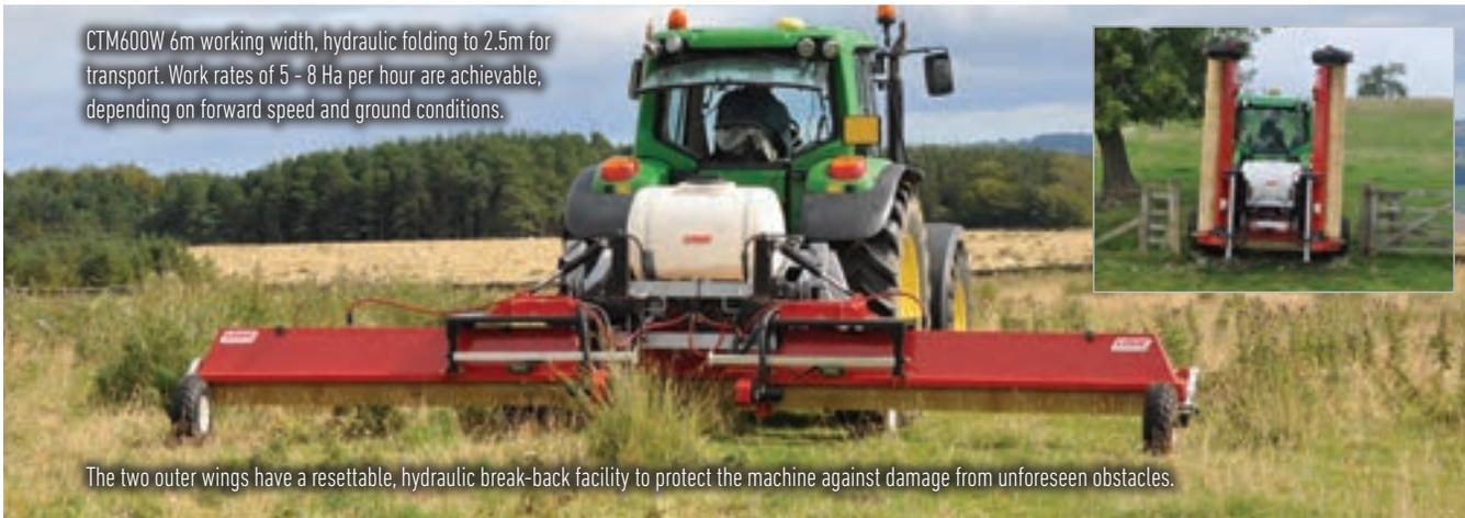
The two outer wings have a resettable, hydraulic break-back facility to protect the machine against damage from unforeseen obstacles.
