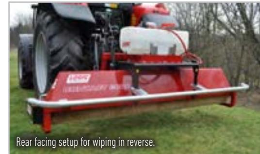
Rear facing setup for wiping in reverse.
