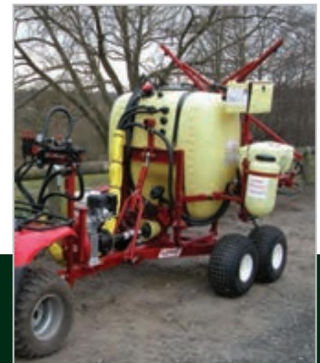
System 40 tandem axle fitted with spreader (left) or with sprayer (above) provide very stable units suitable for rough ground or for very soft conditions. Both applications are shown here with S40T13 models, featuring reverse drive with centrifugal clutch, to provide the same PTO rotation direction as a tractor.
