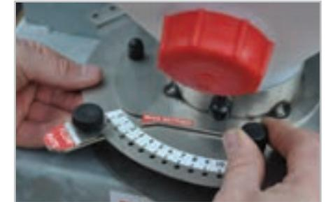
Bias setting: this adjustment is cleverly incorporated into the metering plate, compensating for the different characteristics of each type of product. In this way, even spreading can be consistently achieved.
