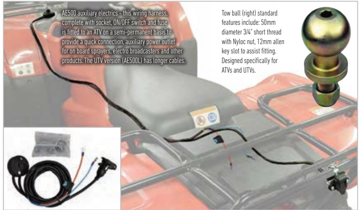
AE500 auxiliary electrics - this wiring harness, complete with socket, ON/OFF switch and fuse is fitted to an ATV on a semi-permanent basis to provide a quick connection, auxiliary power outlet for on board sprayers, electro broadcasters and other products. The UTV version (AE500L) has longer cables.
