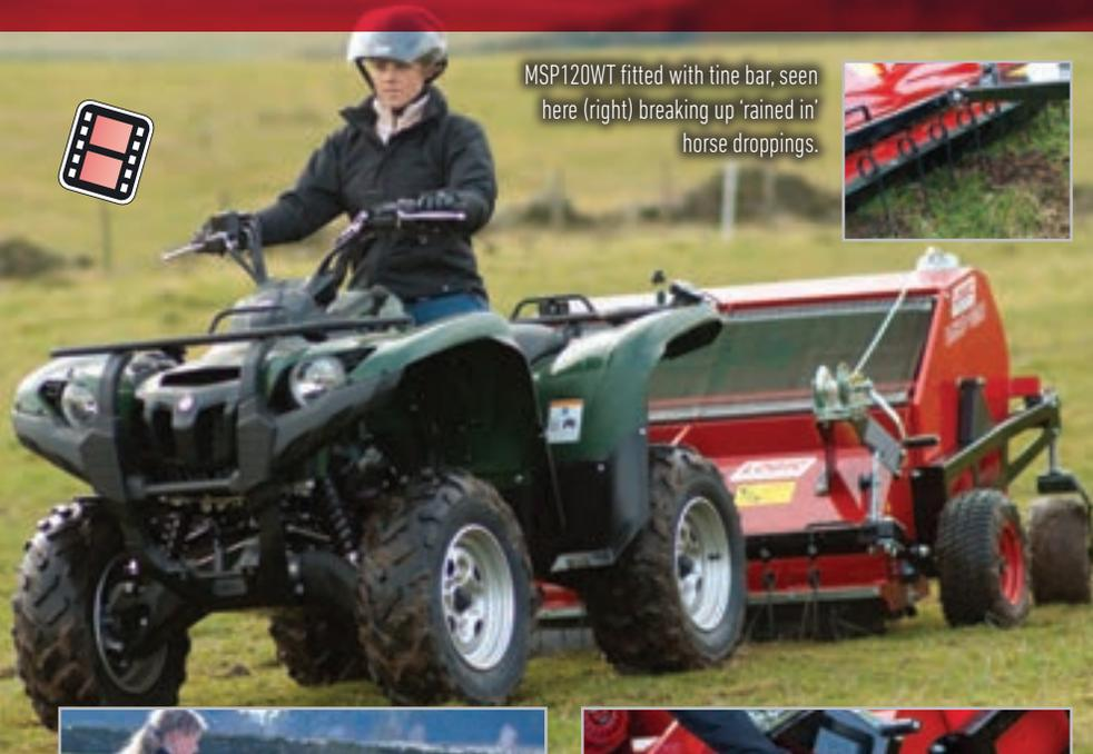
MSP120WT fitted with tine bar, seen here (right) breaking up 'rained in' horse droppings.
