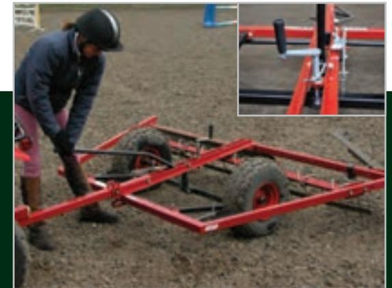
Easily operated over centre lever raises the Pro-Grade for transporting then lowers it into the work position. Inset picture shows the depth adjustment jack to set the blade to the best working level in various surfaces.
