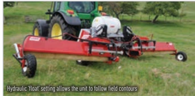
Hydraulic 'float' setting allows the unit to follow field contours
