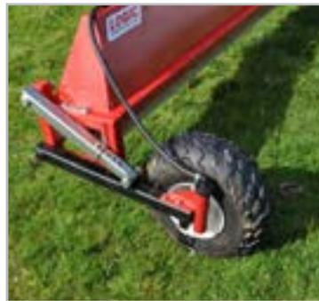
Simple height adjustment gives wiping heights of 400mm down to 50mm. Seen here with optional bout marker fitted to help line of sight and prevention of misses.
