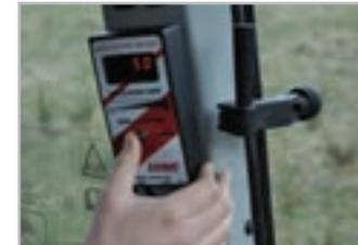
Positioning the supplied control box in the cab close to the driver allows any adjustments to chemical flow rate to be carried out whilst on the move.
