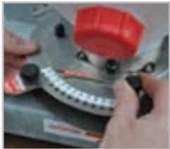
Stainless steel spreading disc with easy bias adjustment. Unique flow control and disc shape to maintain an accurate spread pattern.
