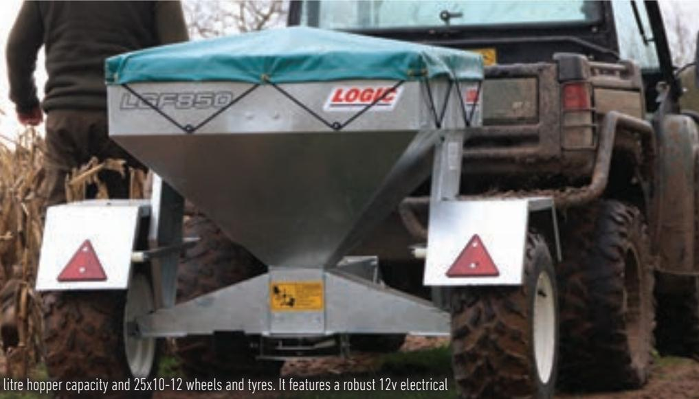
LGF850 trailed game feeder has a 340 litre hopper capacity and 25x10-12 wheels and tyres. It features a robust 12v electrical mechanism with remote ON/OFF control box and stainless steel disc plate which gives a 3.0 metre spread width. This machine is an all-welded one piece monocoque construction which maximises the strength whilst keeping it light to tow. Options of LMF103 mudguards, LMF101 tonneau cover and LMF108 extension sides to 610 litres are available.
