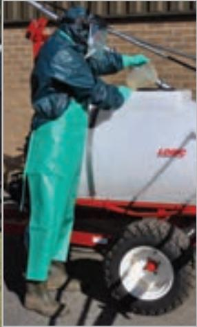
TS400S trailed sprayer with 270 litre capacity tank and a choice of 4.5, 9.0 or 14.4 litres/min pumps to be used with optional booms of 1.5 metres to 4.0 metres, single broadcast nozzle, hand lance and 15.0 metre hose reel.
