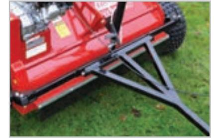
This model has a simplified drawbar and is towed in the central position.
