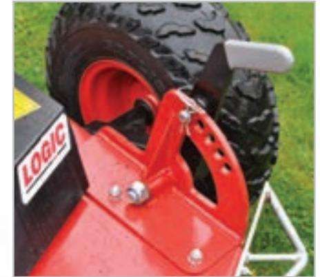
Cutting height adjustment can be carried out simply by moving the spring assisted height lever to one of 5 positions (from 20mm up to 160mm) and securing with the pin and clip.
