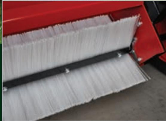
The brush is constructed of 4 banks of sturdy 150mm nylon bristles mounted in a strong frame. It can be raised to a maximum of 300mm using the hand operated jack and is driven by an easy to start Honda 5.5hp engine with centrifugal clutch.
