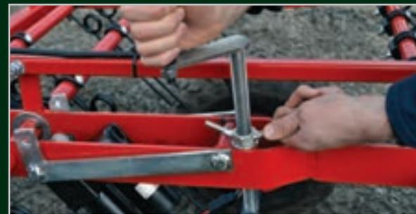
Super Harrow depth control is easily adjusted to provide an accurate setting to suit the type of surface and incorporation requirements.
