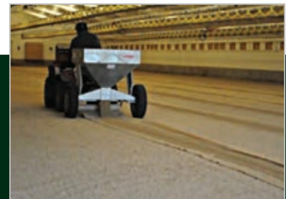
This basic LCF160 lays out approximately 1500kg of feed on 6 rows of paper in this broiler house in 5 minutes (plus filling time) a fraction of the time of previous methods.
