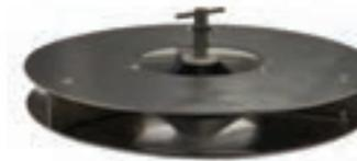
Low impact delivery system - this central cone, unique to Logic machines, reduces the impact of the product hitting the high-speed spinning disc (left). When slug pelleting or spreading fertiliser this minimises 'dusting' (when the product breaks up on impact with the disc). It is also a major benefit when broadcasting seeds, as they are protected from damage compared with some other systems. This leads to higher germination rates.
