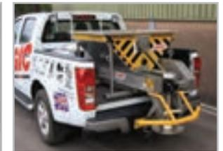
PDS150D can be mounted into any suitable utility vehicle or pickup.
