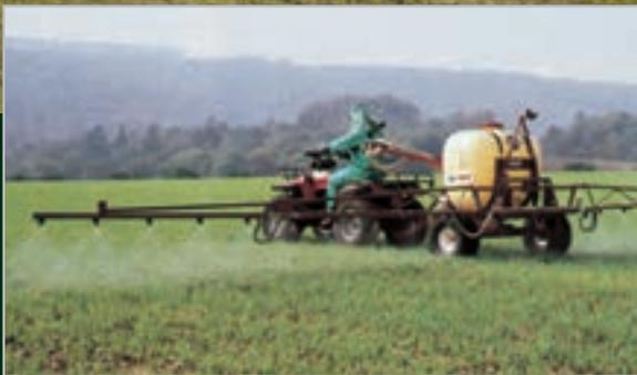
TS500/600 based on the well proven Hardi sprayer, with self-levelling booms of 10.0 -12.0 metre widths. These models are mounted in a sturdy chassis with an engine driven pump providing a stable low ground pressure unit. The sprayer can be mounted on a tractor or as a front tank with adaptor kit for larger sprayers.
