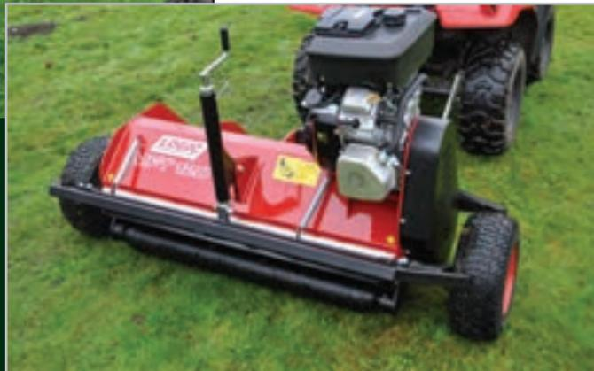
MFT120B18 seen here with standard wheels alongside. The height adjustment jack is spring assisted to make raising this very robust flail mower quite easy.
