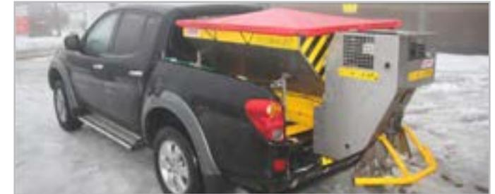
PDS hoppers are manufactured from stainless steel with a capacity of 585 litres (approximately 750kg). The mesh hopper screen, the sluice gate and the deflector vanes which allow salt to be cast to left or right are in common with the GDS range. Optional extras include a PDS208 tonneau cover, quick-attach PDS210 disc shroud and PDS106 flashing beacon.
