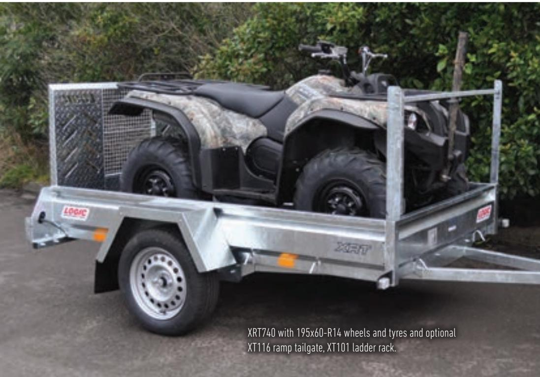
XRT740 with 195x60-R14 wheels and tyres and optional XT116 ramp tailgate, XT101 ladder rack.
