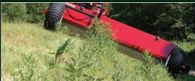
The brush core is especially designed to prevent chemical passing along the length of the brush when used on side slopes.
