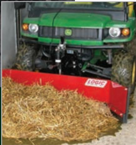
UTS210 yard scraper - suitable for cow sheds, cubicle houses, pig units, poultry houses, etc. With a working width of 1.7 metres, the heavy duty, one piece blade is fitted with replaceable bottom and wing rubber wearing strips. Raise and lower is operated from inside the cab with the remote controlled electrical actuator.
