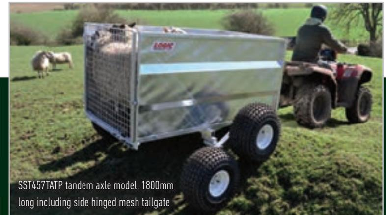
SST457TATP tandem axle model, 1800mm long including side hinged mesh tailgate
