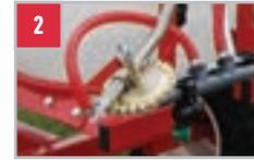
Adjustable break-back clutch for boom safety and protection.
