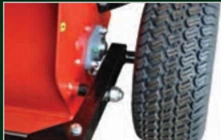
Detail shown here of the brush rotor external bearing which permits a clean operating location and easy access for maintenance.
