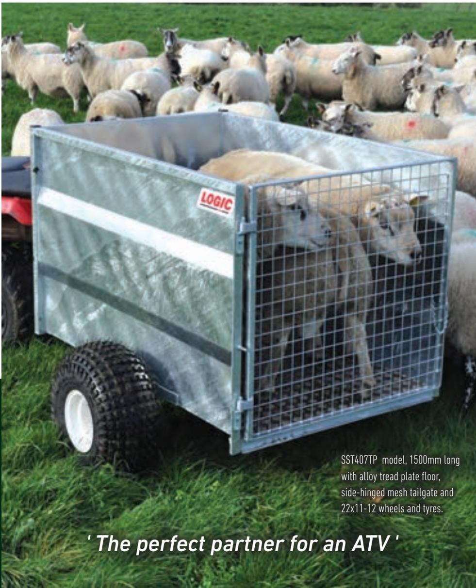
SST407TP model, 1500mm long with alloy tread plate floor, side-hinged mesh tailgate and 22x11-12 wheels and tyres.
