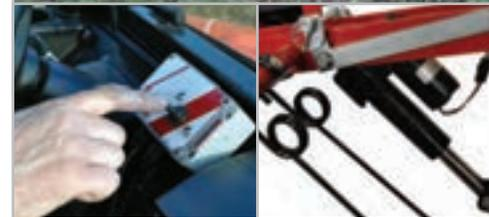
The control box is supplied with ample cable for positioning close to the operator's driving position. This allows it to be used with many types of towing vehicle.
