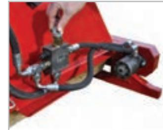
The brush on all tractor mounted models is driven by the hydraulic motor which is easily adjusted using a simple flow control, allowing the operator to set the optimum rotational speed.
