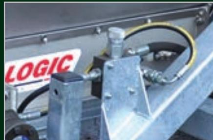
The oil flow control valve (above) allows the operator to select the optimum spreading width for the area being treated, from 3.0 - 14.0 metres.
