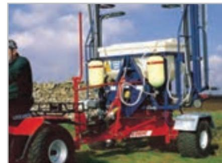
System 40 single axle (above) fitted with an Avadex™ TMA4 applicator to provide an ultra-low ground pressure unit for use in soft conditions.
