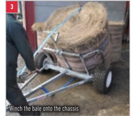
3 Winch the bale onto the chassis
