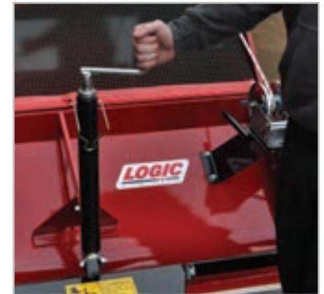
Raise and lower is adjusted by turning the screw jack handle which offers very fine adjustments. This gives a very accurate height control of the brush which is good for all surfaces, particularly short, fine piles.
