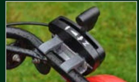
The remote throttle gives control from the operator's driving position.
