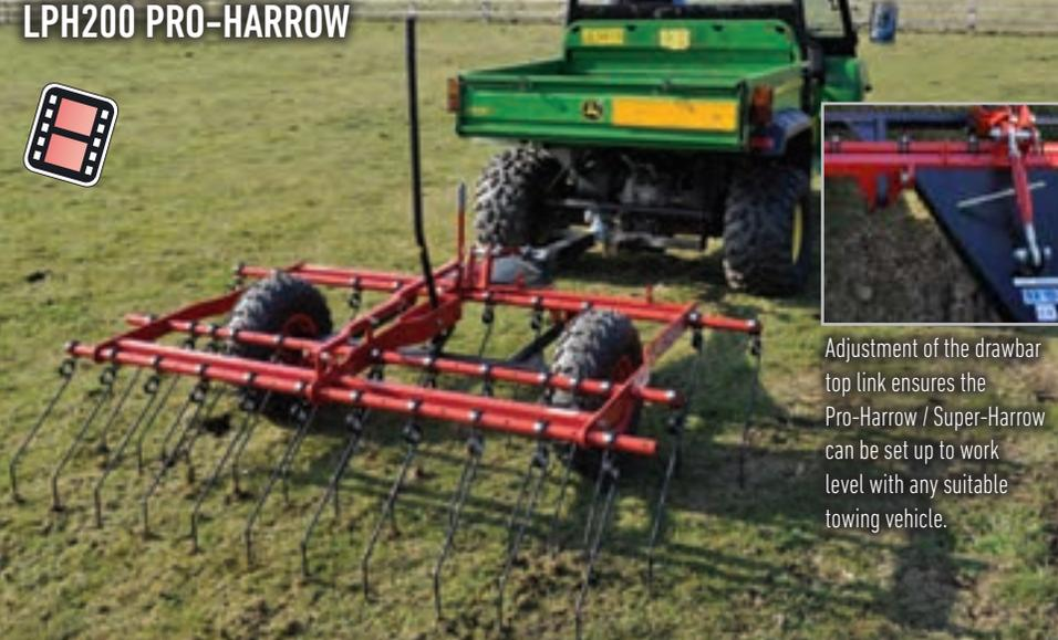
Adjustment of the drawbar top link ensures the Pro-Harrow / Super-Harrow can be set up to work level with any suitable towing vehicle.
