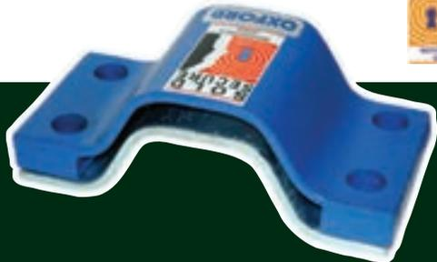
ATV116 block ground anchor - this 'block' is useful in high traffic areas as its low profile allows it to be driven over without damage. The double thickness hardened steel makes it very difficult for the block to be breached. Once attached, the bolt heads are rendered useless to prevent extraction.
