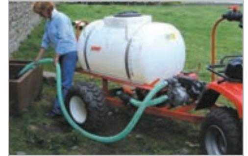
SLB620H has a Honda 2" diameter pump for discharge into elevated tanks or troughs. With a powered pump there is also an optional 5.0 metre suction hose kit which allows you to "self-fill" the bowser from any available fresh water source.
