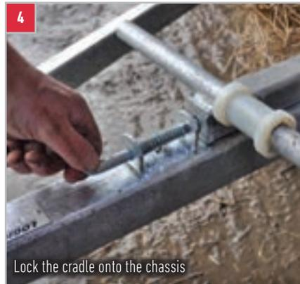
4 Lock the cradle onto the chassis
