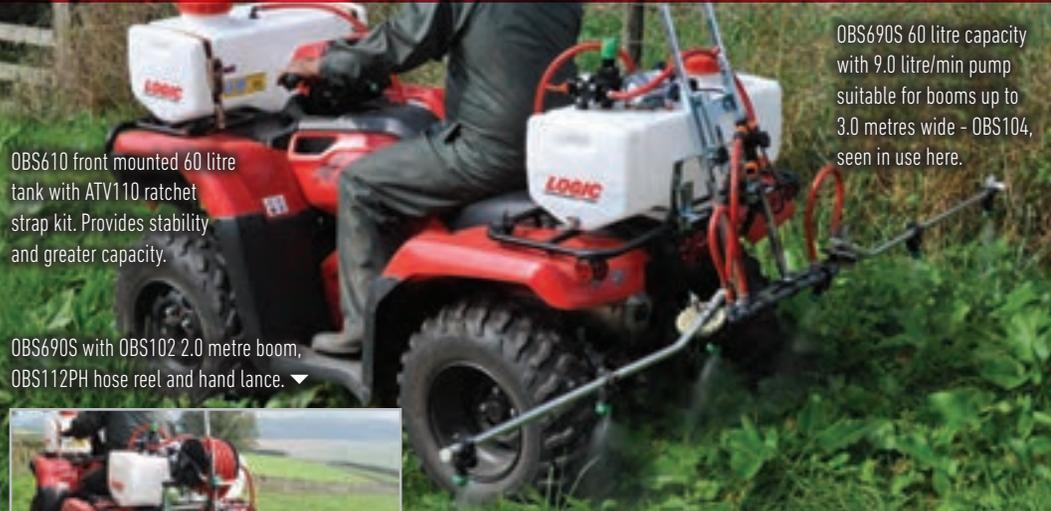
OBS610 front mounted 60 litre tank with ATV110 ratchet strap kit. Provides stability and greater capacity.
