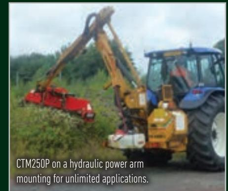
CTM250P on a hydraulic power arm mounting for unlimited applications.
