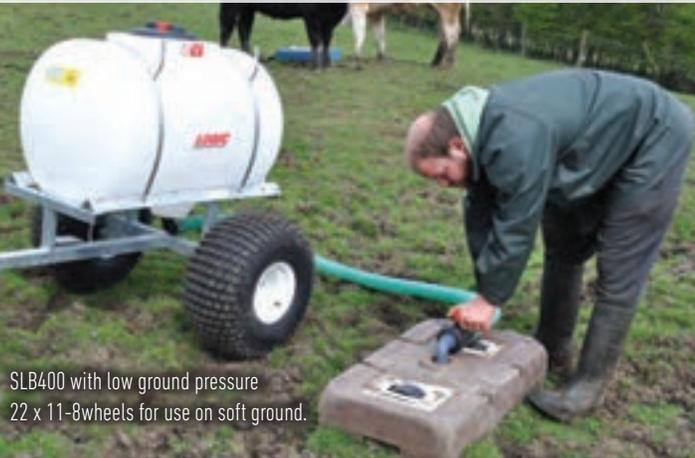
SLB400 with low ground pressure 22 x 11-8wheels for use on soft ground.
