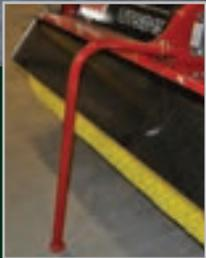
UTS215 parking leg - allows the power brush to be stored without the bristles taking any weight therefore preventing distortion of the brush. This prolongs the life of the brush bristles and permits more stable parking.
