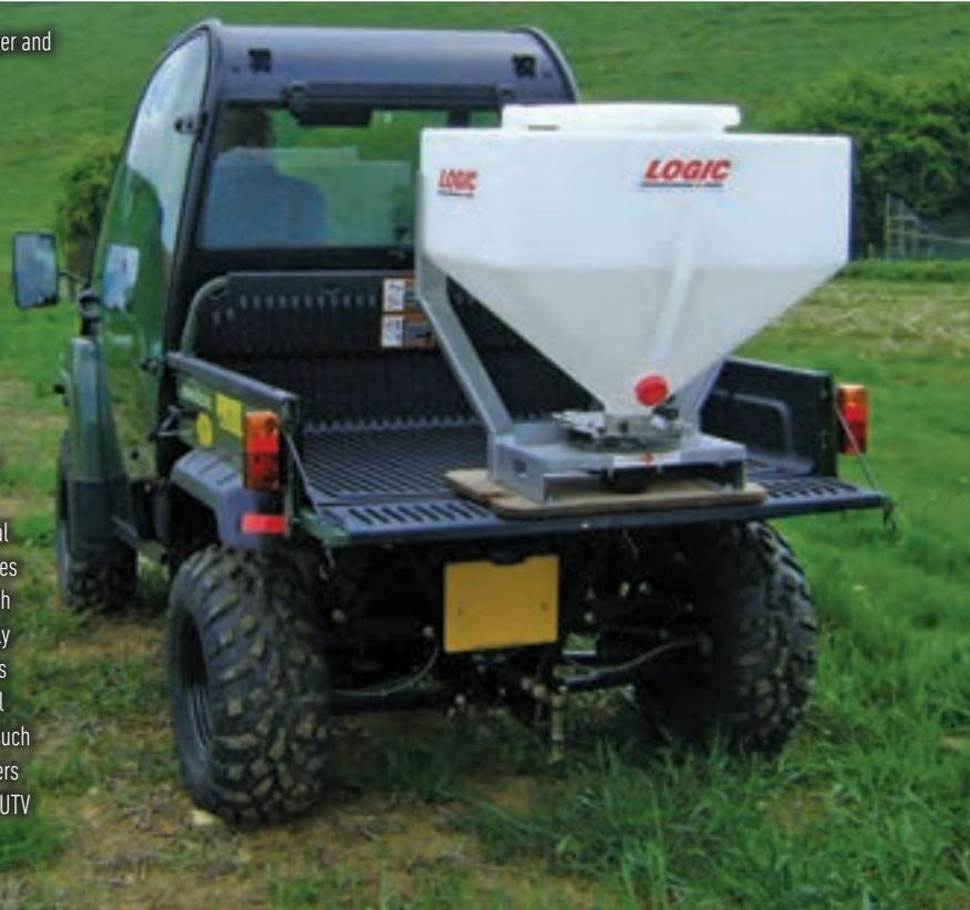
The range has two motor sizes. The EBC-TFL80 range uses a motor with a power demand that is compatible with most ATV electrical systems. The EBC-TFL120 range uses a significantly up rated motor which is capable of delivering consistently wider spread widths; this range has been designed to suit the electrical systems found on larger vehicles such as tractors or self-propelled sprayers and is therefore recommended for UTV use (see chart below).
