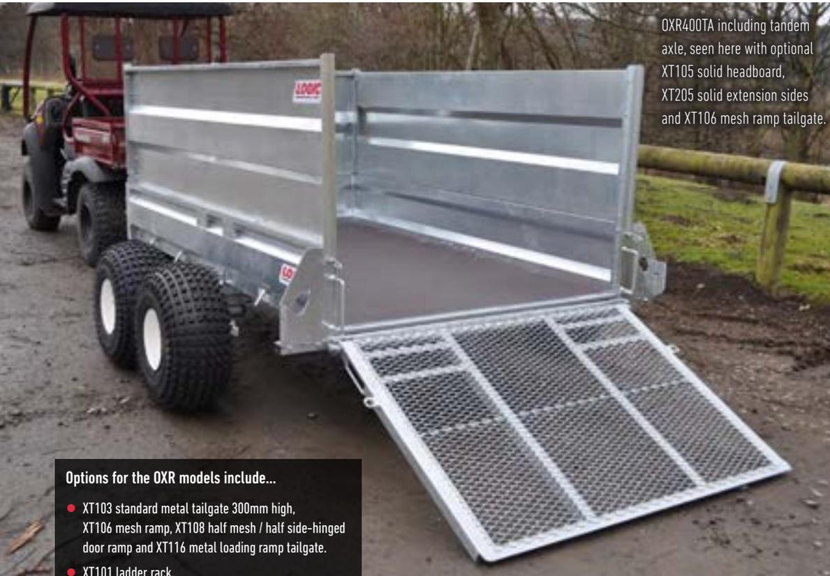
OXR400TA including tandem axle, seen here with optional XT105 solid headboard, XT205 solid extension sides and XT106 mesh ramp tailgate.
