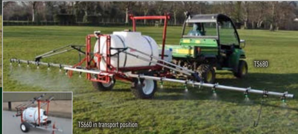
TS660/680 sprayers feature the same strong, rotationally moulded, translucent, polyethylene 600 litre tank, mounted on a sturdy 'A' frame chassis with low ground pressure 23 x 10.5-12 wheels and tyres. Output is supplied from a Honda engine, 25 litre/min diaphragm pump controlled by remote electric ON/OFF and manual pressure regulation. A 15 litre clean water tank is mounted to comply with Health & Safety regulations.
