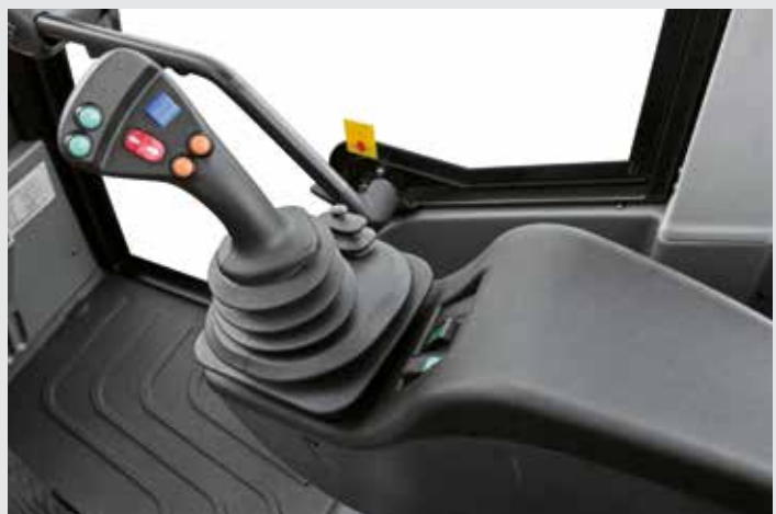
The arm-rest and joystick form a unit with the seat and maintain their position in relation to the operator whatever movement the seat makes. Perfect ergonomics!
