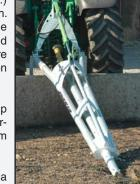
A triangular structure, which is made up of two side tubes and an upper one, makes the machine highly stable. Furthermore, the intersection point of the tubes prevents the transmission shaft from bending.
