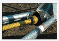
The Jumbomixer is standard fitted with a reinforced P.T.O.-shaft in star-shaped tube with 1 3/4" shaft and shear bolt. A power of 100 HP minimum is required. The total length is 7 m and the weight
