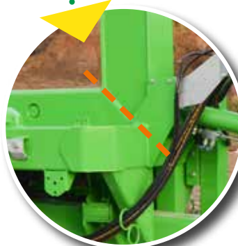
Design of the telescopic arm with diagonal welding and reinforcement, which makes it way stronger.
