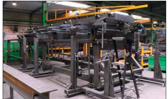
The jigs used in the factory ensure precision and rapidity during the manufacturing process
