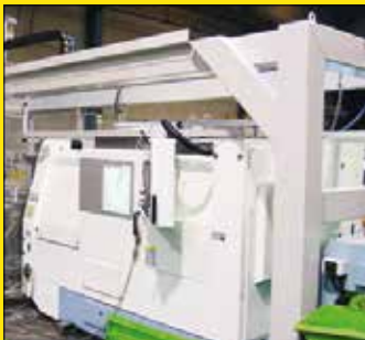
Lathe with digital control
