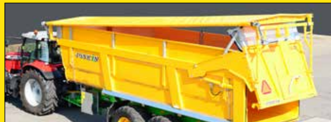
TELECOVER cover compatible with the hydraulic extensions
