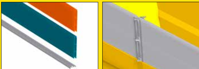
Interlocking system of the alu extensions
