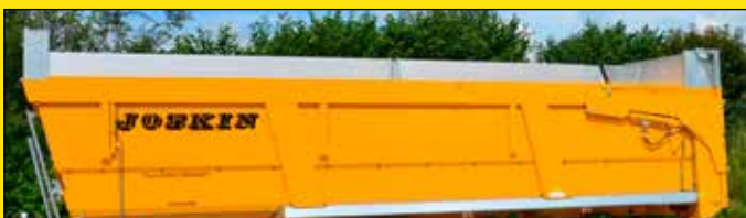
Combination of alu extensions and a hydraulic steel extension (50 cm)
